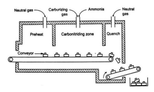
Suitable for plain carbon steels such as small gears, bolts, nuts, pins etc.
