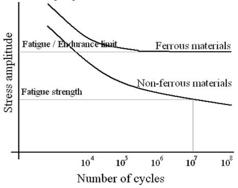
**Endurance ratio** – ratio of fatigue stress to tensile stress of a material. For most materials it is in the range of 0.4-0.5.
