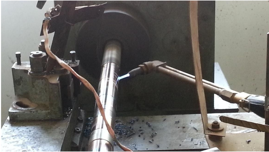
Fig. 4.4: Torch heating the workpiece
